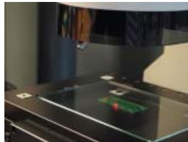
Light spot to indicate the current measuring position (activated for a short time during stage movement)
